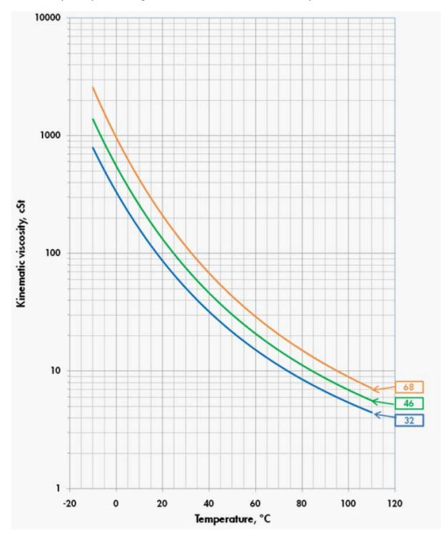
Viscosity – Temperature Diagram for FluidForce Vane 2000 hr Warranty Lubricant VAWO2000-xxGT
